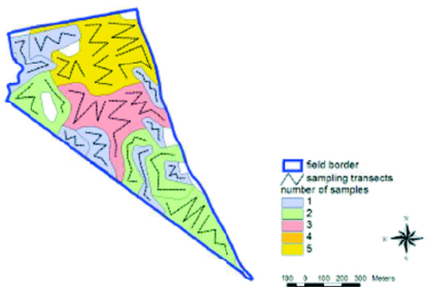
Fig. 5. Layout of improved soil sampling scheme for a 75 ha field near Baborówko, showing field borders, borders of soil polygons, and possible walking transects for sampling, applying a buffering operation of 15 m around all polygon borders and first and second rule for determining the numbers of samples in each polygon (see text for details on the procedure)
