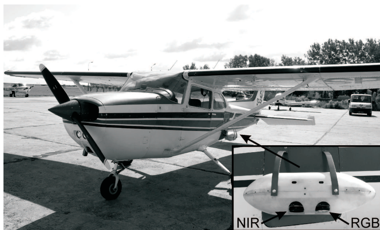
Fig. 1. Multispectral sensor system for low-altitude remote sensing (MSS-LA-RS) mounted on a Cessna plane.
